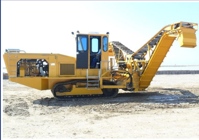
250 tph Durrant 566-70 salt harvester
