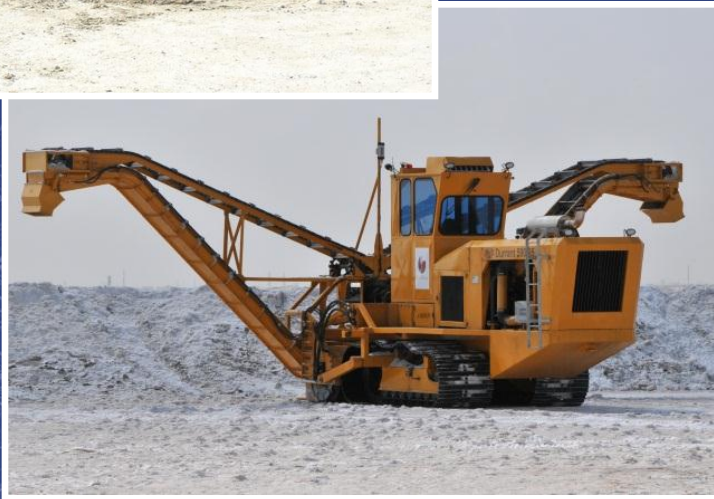
350 tph Durrant 590-95 salt harvester
