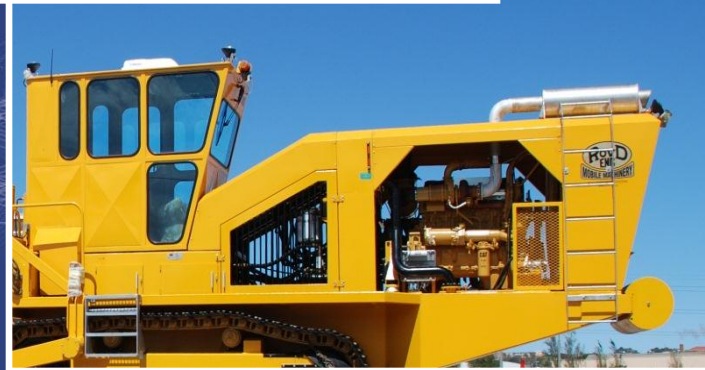
450 tph Durrant 7160-120 salt harvester
